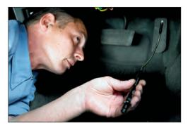
Features a high-intensity white LED and a 7" cable (providing 14" of reach) that allows you to see into the tightest spots. IPX4 rated for water-resistance. Pocket clip.
